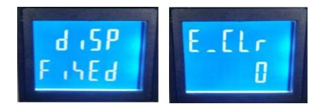
1.3 Cycle display the device information Press "FUNCTIONAL BUTTON" enter into operation page 7th, press "SELECT", the letter "d" will flash, press "SET" again enter into cycle display mode. See as follows:
